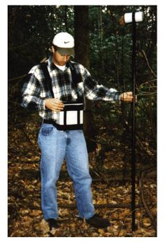
standard GEM capabilities: the Walking Mag option that enables the operator to sample while walking. Having nearly continous data on survey lines also helps to incre-ase the accuracy of interpretations.
